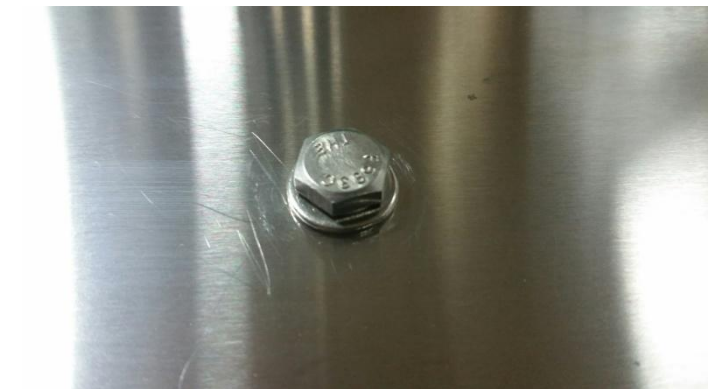
Drill a hole in the top of the hood on the left hand side, 5.125" from back, 2.875" from side of hood Hole is for a 1/4" bolt, use a 9/32 (.281") drill for easier fit, seal bolt with flat washer.
